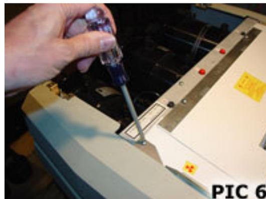
The plate aligns the tubes with small pins facing down, these can bind a little so pry up just under the plate with a screwdriver if needed. (see **PICs 7 and 8**)
